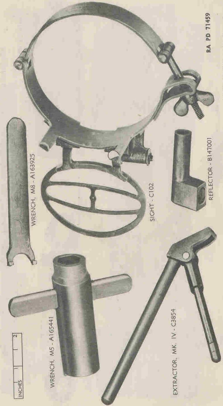
Figure 6—Accessories for Gun, Machine, Cal..30, Browning, M1917 and M1917A1; and Mount, Tripod, Machine Gun, Cal..30, M1917A1
